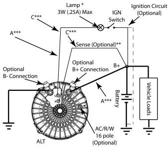
Alternator is self excite. For basic operation B+ and B- needs to be connected. All other connections are optional.
