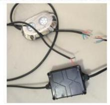
3, Connect the control box to the 12V DC power, (12V battery),
