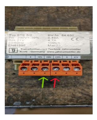
Please ensure that the input power cable is connected to the clamp with the red arrow (+10%). If it is installed on the clamp with the green arrow (230V) please remove and switch to the clamp with the red arrow (+10%)
